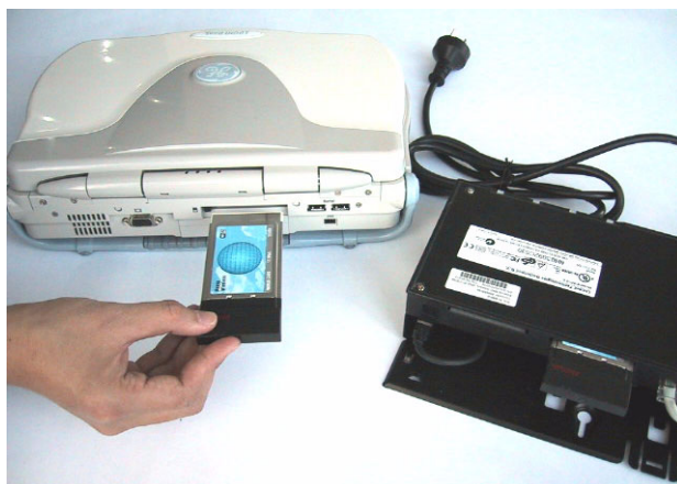
Figure 3-10. Wireless LAN Connection
